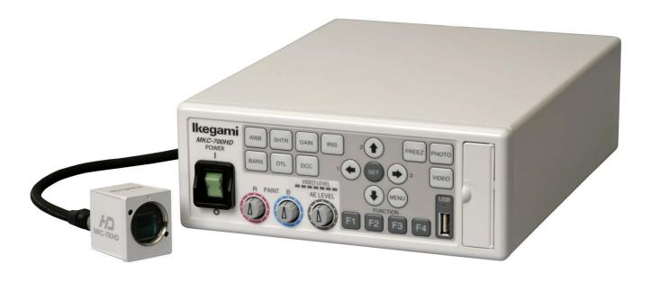
Employs full HD (1920 x 1080) 3CMOS sensors for the highest image quality (horizontal resolution 1,000 TVL, S/N 56dB) and two times higher sensitivity compared to conventional models (2,000lx/F16:LINE MIX ON), also a newly developed digital processor giving a high grade picture output. Auto image correction provides a higher contrast image without halation or black defects.
